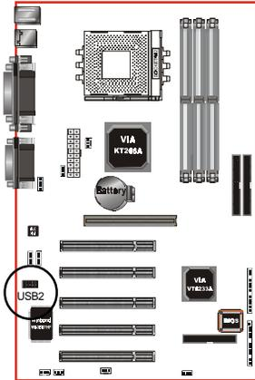
**USB2:** USB port header pins for share with four USB ports.
