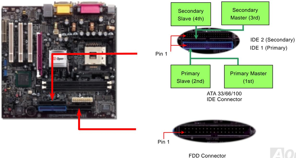
IDE1 is also known as the primary channel and IDE2 as the secondary channel. Each channel supports two IDE devices that make a total of four devices. In order to work together, the two devices on each channel must be set differently to **Master** and **Slave** mode. Either one can be the hard disk or the CDROM. The setting as master or slave mode depends on the jumper on your IDE device, so please refer to your hard disk and CDROM manual accordingly.
