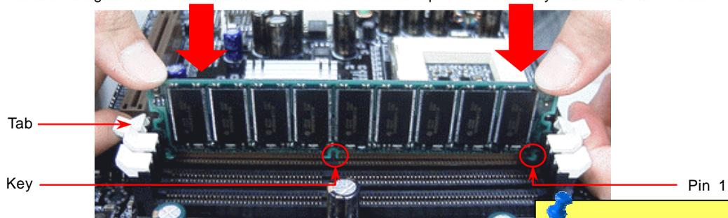
3. Repeat step 2 to finish additional DIMM modules installation.
