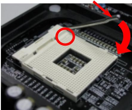
2. Locate Pin 1 in the socket and look for a cut edge on the CPU upper interface. Match Pin 1 and cut edge, then insert the CPU into the socket.
