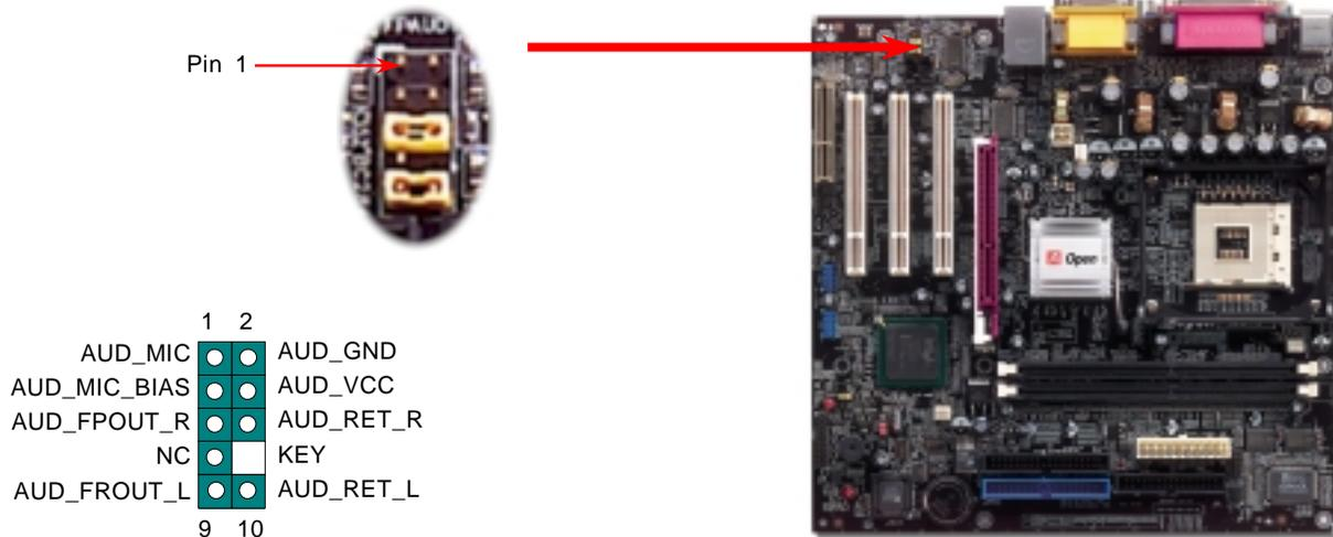
**Note:** Please remove the jumper cap from the Front Panel Audio Connector before you connect the cable. Do not remove this yellow jumper cap if housing without an audio port on the front panel.
