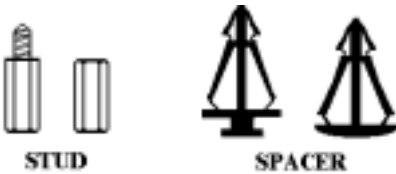
Figure 2-3. The outline of stud and spacer
