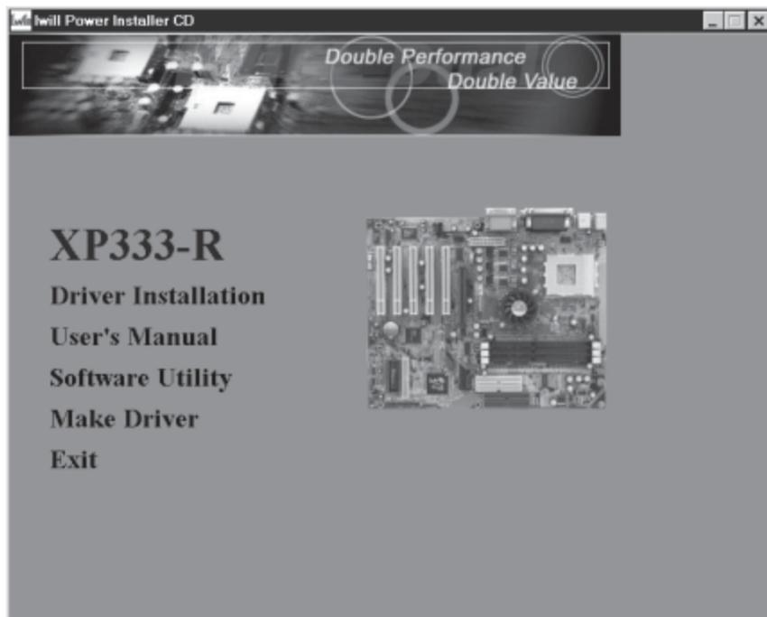
Install the first item for the Ali chipset by clicking on it and following the install program instructions. Make sure you install this before you install any other software on the disc. If you will use an ATI Rage 128 Pro display card, also install the “Patch Driver”.
