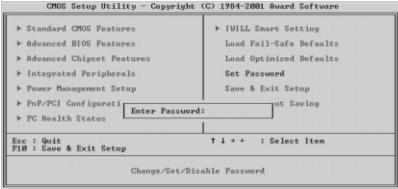
These items are used for setting passwords. When a password is set and the Security Option field in Advanced BIOS Features is set to Setup, you will be required to enter the password every time you try to enter the CMOS Setup Utility. This prevents an unauthorized person from changing any part of your system configuration. Additionally, if the Security Option field is set to Boot, the BIOS will request a password every time the system boots. This prevents unauthorized use of your computer.
